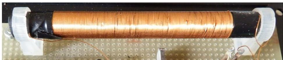
On both ends the coil is fixed with tape. The antenna is mounted in two plastic holders onto the PCB.
