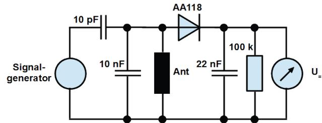
From the resonance frequency  $f_{res}$  the inductance of the coil can be calculated:
