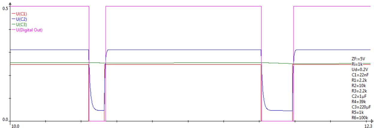
The voltage on the first capacitor, after rectification of the IF, decreases and increases very fast. Its small capacity of 1 µF has no relevant influence and just smoothes down the 455 kHz peaks from the rectifier diode.
